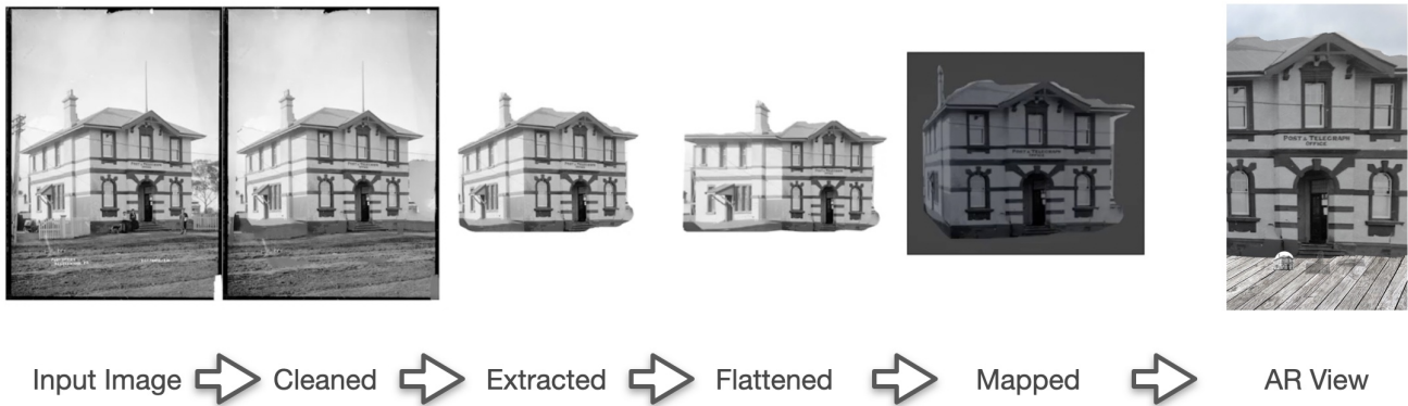
Figure 2: ARephotography aims to combine the concept of rephotography and Augmented Reality (AR) to create experiences where one can view historical buildings as they once looked. Our approach takes a historical photograph (Left) of a building and produces a textured 3D model that can be placed in AR over the current view of the building (Middle and Right). Original photograph: Green & Colebrook (Firm). Ngaruawahia Post Office and mail coach, 1910 - Photograph taken by G & C Ltd. Price, William Archer, 1866-1948 :Collection of post card negatives. Ref: 1/2-001602-G. Alexander Turnbull Library, Wellington, New Zealand. /records/23009835
