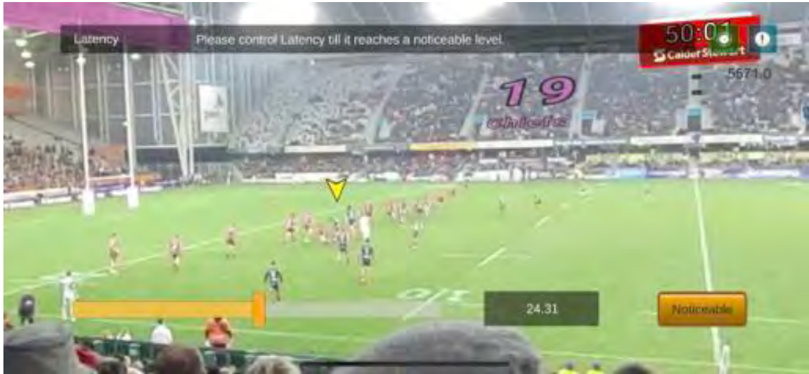
Figure 5.6: Our user study prototype showing the latency factor delayed by 24 frames (1 second) controlled by the slider at the bottom. Optimally, the arrow should point at the referee (in white outfit).
