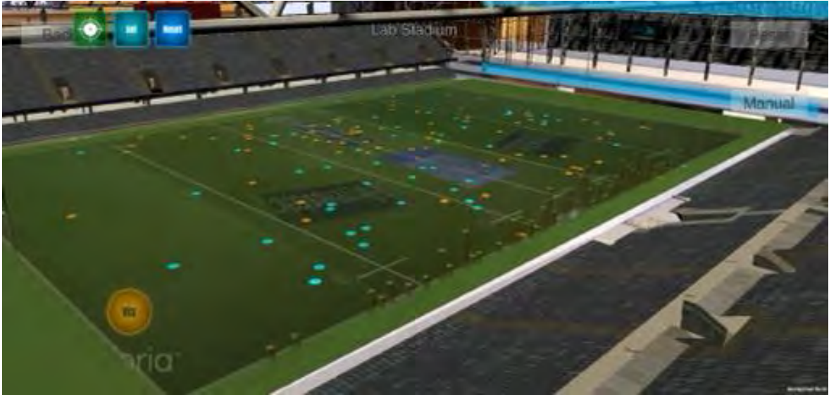
Figure 3.7: Miniature lab AR prototype to evaluate visualizations from a third-person perspective. Shown is a virtual stadium overlaid on a A0-sized printed field.
