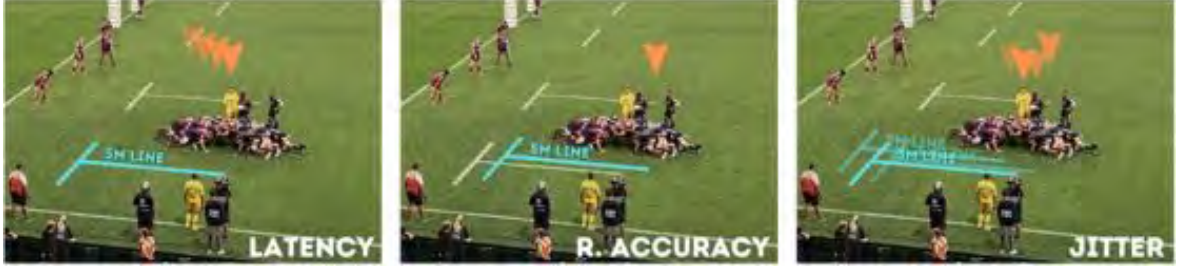
Figure 5.2: An illustration of technical factors evaluated: latency, registration accuracy, and jitter. Visualizations are shown in blue (static) and orange (dynamic) where the arrow is targeting the person in yellow.
