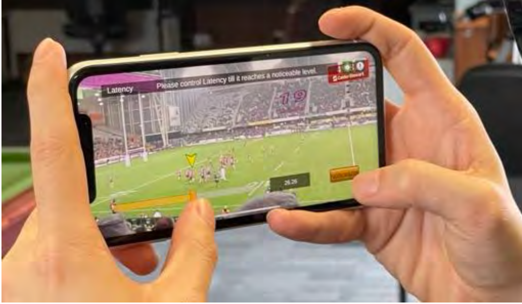
Figure 5.4: User study session where a participant controls a slider to manipulate the technical factor. The goal is to set the slider until they obtain the noticeable and disruptive levels. Shown in the image is latency.
