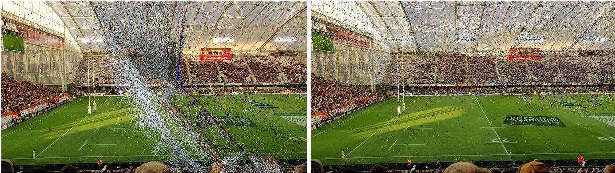
Fig. 6. Visualization of 3D point cloud overlaid onto a camera image (from the crowded dataset) using the computed camera pose. Left: Visualization using camera pose computed by one expert. This image is considered to be not correctly localized with an average reprojection error above 500pixel. Right: Visualization using camera pose computed by ten experts. This image is considered to be correctly localized with an average reprojection error of 8.9 pixel.
